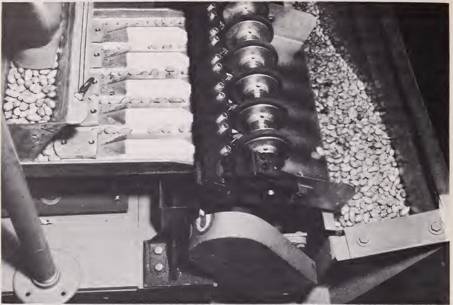
FIGURE 19.— This machine cuts the skins longitudinally on individual kernels preparatory to water blanching.
